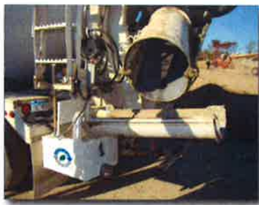
Figure 7. Chute washout box
