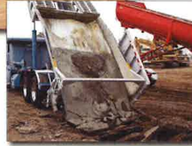
Figure 15. Delivering hardened Concrete to a recycler
