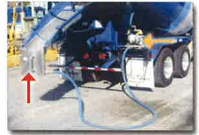
Figure 8. Chute washout bucket and pump
