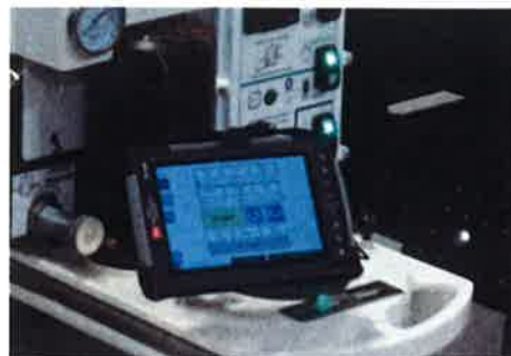
The ruggedized TC-100 handheld computer / wireless controller / datalogger provides intuitive remote exerciser control
