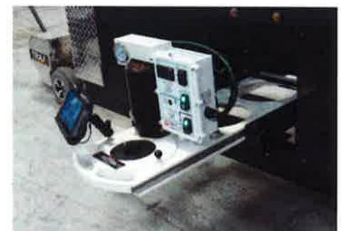
Optional TM-7 HD Plus valve operator provides 2500 ft-lb of torque for turning large valves
